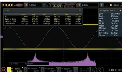
Perform TIE measurement on the clock signal with the jitter and make an analysis on the measurement results through trend graph and histogram.
