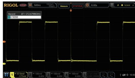
Adopt the segmented storage technology, you can set the trigger conditions to make a selective choice in capturing and saving the signals that you are interested in
