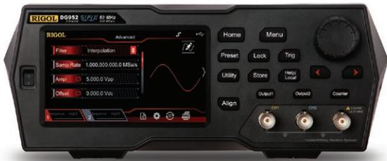
As a multi-functional signal generator, DG900 series function/arbitrary waveform generator integrates many instruments into 1, such as function generator, arbitrary waveform generator, noise generator, pulse generator, pattern generator, harmonic generator, analog/digital modulator, and frequency counter. The brand new appearance and user-friendly interface design bring you excellent user experience.
