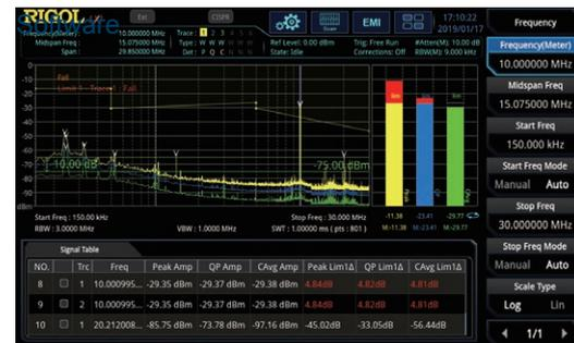
The RSA5000's built-in EMI pre-test application software, combined with CISPR-compliant filters, pre-tests the product for conduction and radiation to identify and improve its conduction/radiation disturbance source and accelerate time-to-market.
