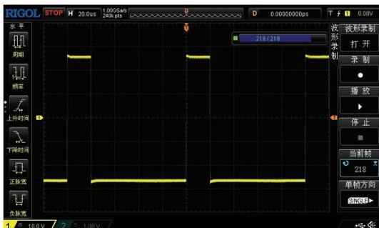
Provide waveform recording option, record waveform changes, playback the waveforms easily, and locate the faults accurately.
