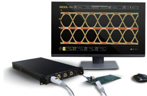
A single device with peripherals can meet traditional oscilloscope applications: connect the display device through the HDMI interface to view the user interface, connect the mouse through the USB Host interface to click and drag, and connect the keyboard to set numbers or strings.
