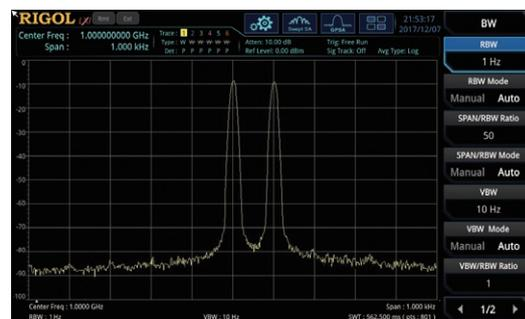
Resolving signals with similar frequencies is critical to verifying many RF devices and systems. With the RSA3000, the RBW resolution bandwidth with a scan bandwidth of only 1 Hz allows you to view more details of adjacent signals.
