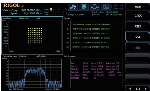
The VSA supports a variety of digital modulation formats such as QAM, PSK, MSK, ASK, FSK, etc. This function is used to quickly demodulate and display multi-dimensional data such as its constellation, eye diagram (baseband signal), spectrogram, demodulation data, etc., to discover problems in the design.
