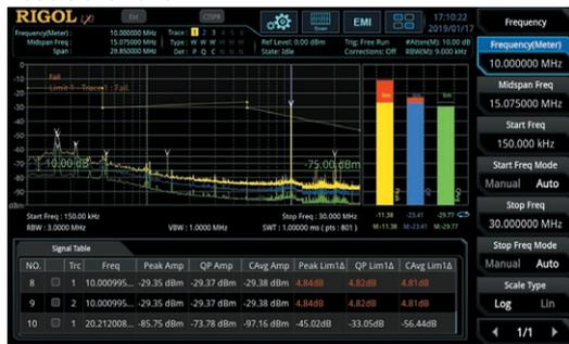
The RSA3000E's built-in EMI pre-test application software, combined with CISPR-compliant filters, pre-tests the product for conduction and radiation to identify and improve its conduction/radiation disturbance source and accelerate time-to-market.
