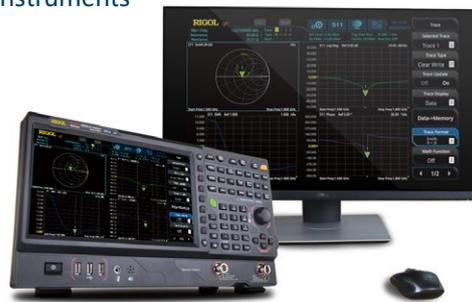
The instrument can be connected to a larger display/monitor via the HDMI interface for better display effects. The Web Control function allows you to directly control the device by accessing the device IP address, improving the experience of remote control.
