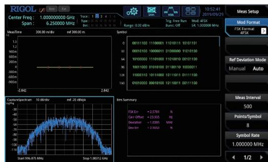
ASK/FSK demodulation analysis software can help engineers demodulate and analyze signals such as TPMS, PKE/RKE, and obtain parameters of signal modulation quality to help products get listed quickly.
