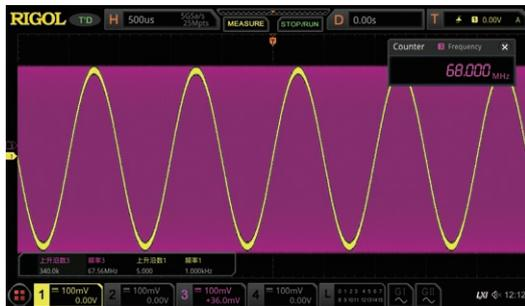
Measure accurate frequency value of the waveforms based on memory, not the screen display.
