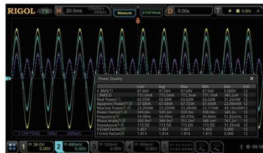
DS8000-R, MSO8000series, MSO/DS7000 series and MSO5000 series oscilloscopes support the optional built-in power analysis software, which can complete the power quality analysis and ripple analysis. The power analysis software can help engineers analyze the commonly used power parameters rapidly and accurately, without needing to make tedious configurations manually or do complicated formula calculation.
