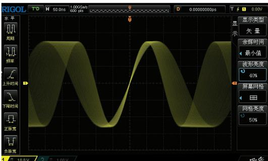
The intensity graded color display capability provides the fluorescent display effect, making the waveform changes obviously to be seen.
