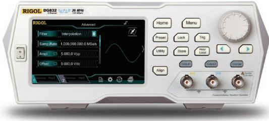
As a multi-functional signal generator, DG800 series function/arbitrary waveform generator integrates many instruments into 1, such as function generator, arbitrary waveform generator, noise
