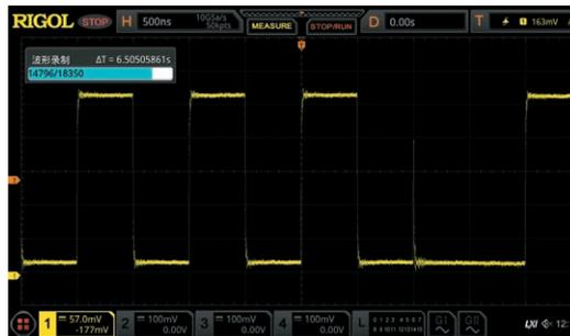
Based on segmented storage technology, deep memory not only ensured the high capture efficiency, but also prolonged the overall observation time for the waveforms.
