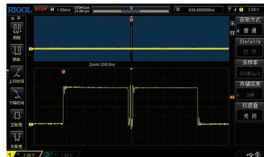
Standard 24M memory depth. It allows users to give full consideration to the overall situation and details of the waveforms, maintain the highest sampling rate for a long period of time without missing any waveform changes.
