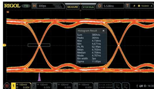
To better observe the transmission quality of the digital signal and understand the Inter-Symbol Interference in the system, so that you can make improvement in the system design.
