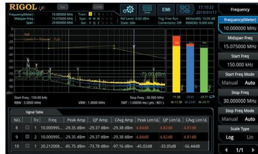
The RSA3000's built-in EMI pre-test application software, combined with CISPR-compliant filters, pre-tests the product for conduction and radiation to identify and improve its conduction/radiation disturbance source and accelerate time-to-market.
