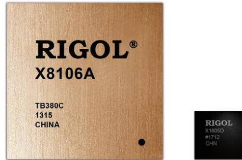
MSO/DS7000 Series Digital Oscilloscope adopts RIGOL's self-developed ASIC chip for digital oscilloscope, which can gain the data acquisition capability of up to 10 GSa/s real-time sample rate, realizing the high integration of all the function modules required for the analog front-end(AFE), and greatly improving the consistency and reliability of the digital oscilloscope.
